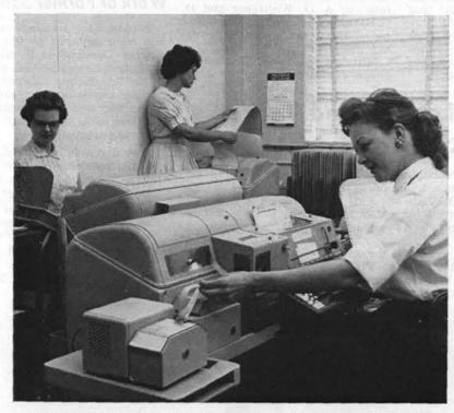
28ASR TELETYPEWRITERS are used to transmit purchase requisition data to purchasing from ordering organizations through the medium of paper tape. Wanda Cupp and Glenna Mosely, foreground and left, operate Teletype transmitters while Juanita Van Jelgerhuis, center, examines a reply at Teletype receiver.
